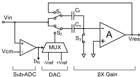
Fig. 3 Switched-capacitor implementation of conversion stage.
