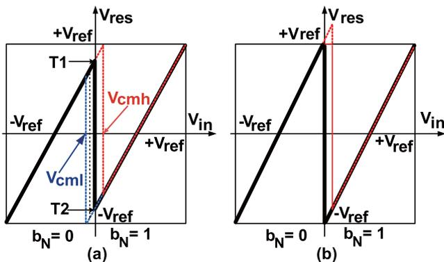
Fig. 2 Transfer characteristic of the conversion stage. (a) radix =  $\beta < 2$ . (b) radix = 2.
