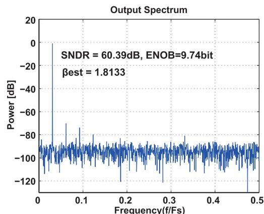
Fig. 14 Output power spectrum of cyclic ADC in chip B with estimated  $\beta$ .
