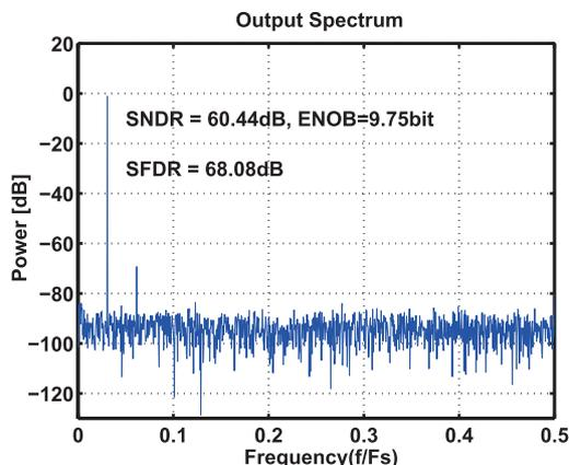
Fig. 10 Output power spectrum of cyclic ADC in chip A with estimated value of  $\beta$ .
