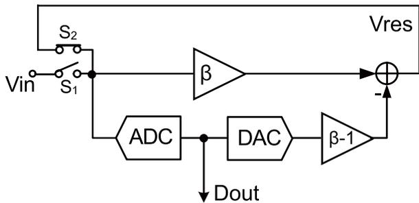
Fig. 1 Simplified block diagram of the non-binary cyclic ADC based on  $\beta$  expansion.
