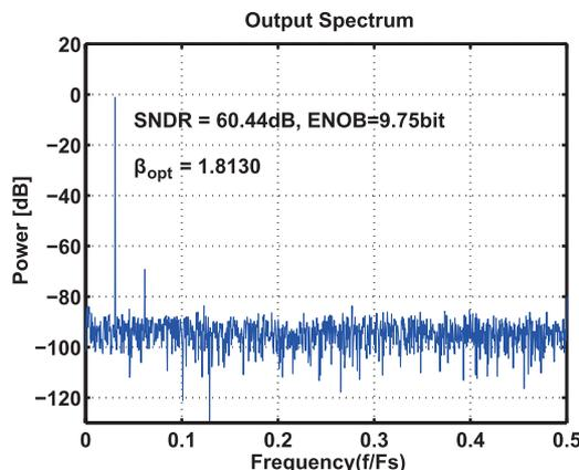
Fig. 12 Output power spectrum of cyclic ADC in chip A with optimum  $\beta$ .
