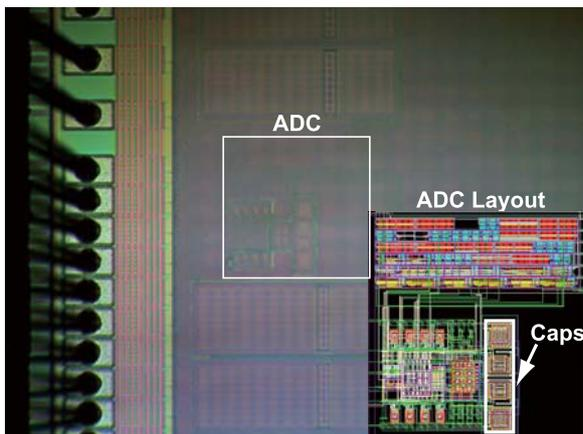
Fig. 8 Chip B micrograph and layout.
