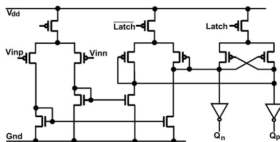
Fig. 6 Schematic of latched comparator.
