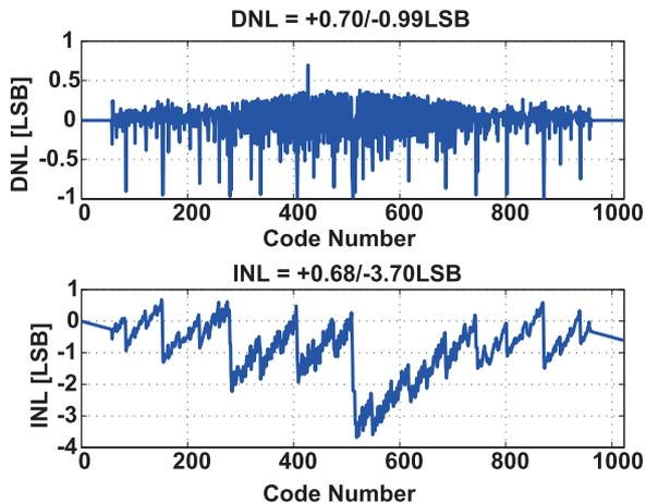
Fig. 15 Measured DNL and INL with designed radix value of chip B.
