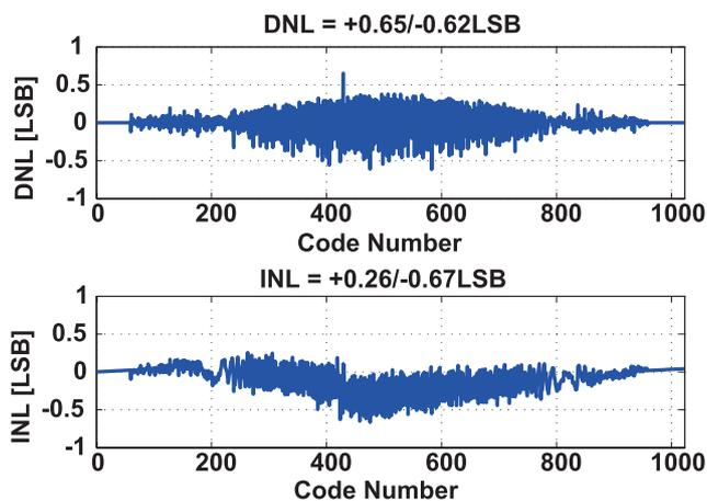
Fig. 16 Measured DNL and INL with estimated radix value of chip B.
