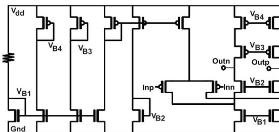
Fig. 5 Schematic of a single-stage folded-cascode amplifier.
