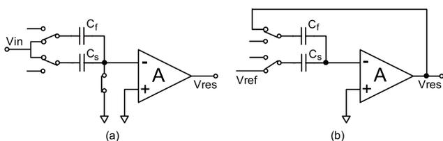
Fig. 4 Switched-capacitor multiply-by- $\beta$  amplifier. (a) Sampling phase. (b) Amplifying phase.
