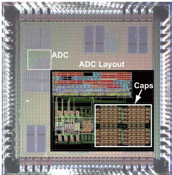
Fig. 7 Chip A micrograph and layout.
